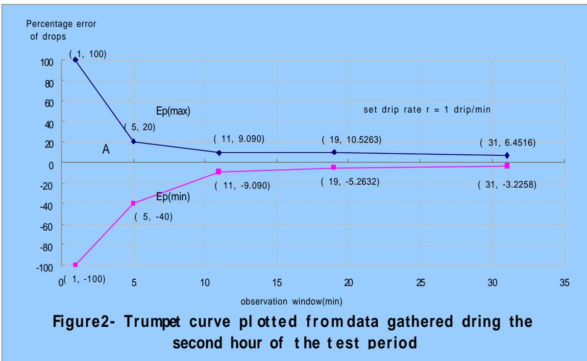
Figure 2- Trumpet curve plotted from data gathered during the second hour of the test period
