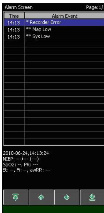
Under the screen, you can view each alarm event including its data, time and the parameters leading the alarm.
